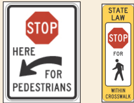
Signage should be used to raise awareness of “stop for pedestrian laws” at intersections along Downtown Streets Images courtesy of USDOT, MUTCD
