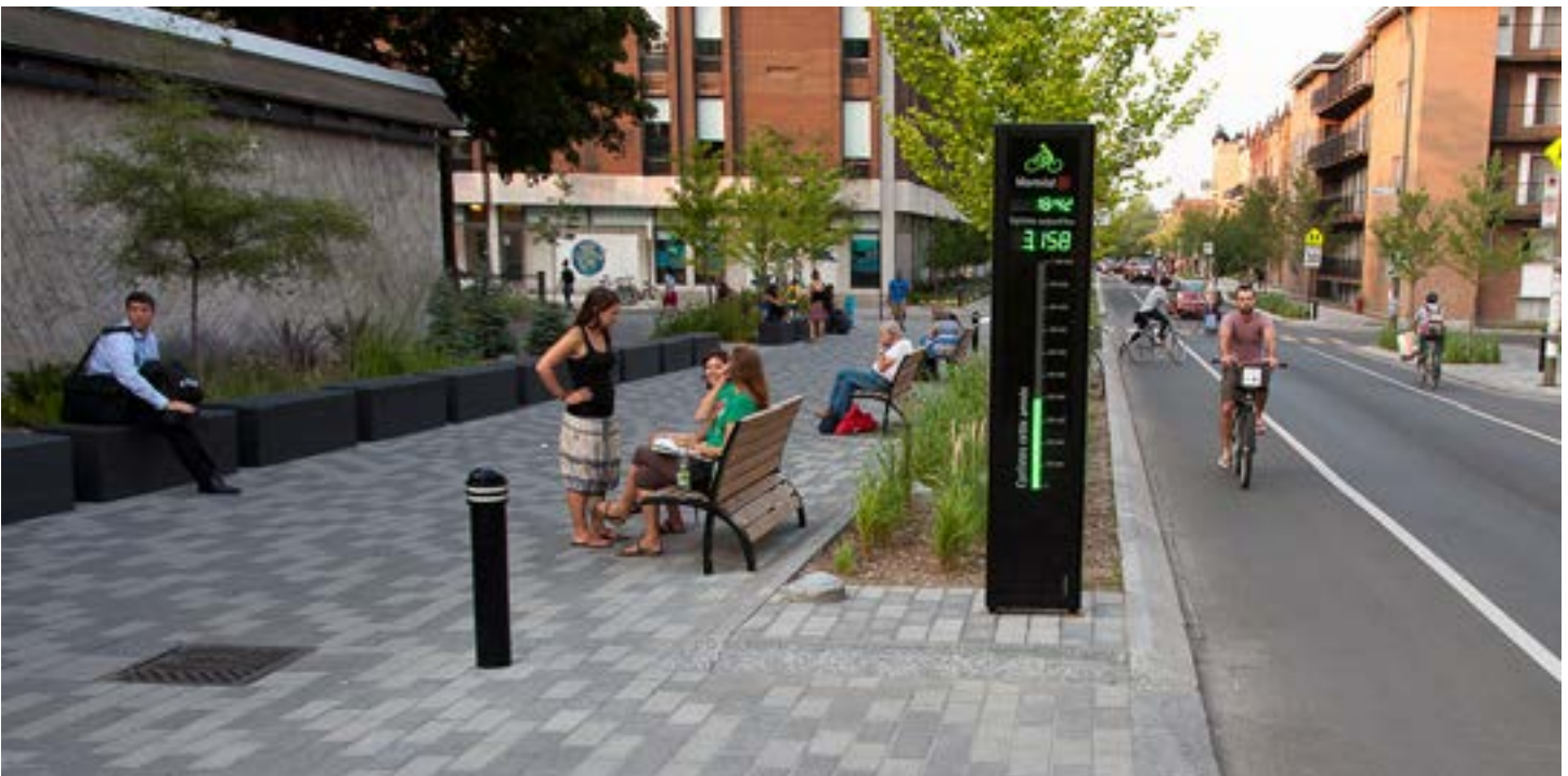
A pedestrian and bike counter placed curbside to measure traffic and activity in a neighborhood in Copenhagen, Denmark.
