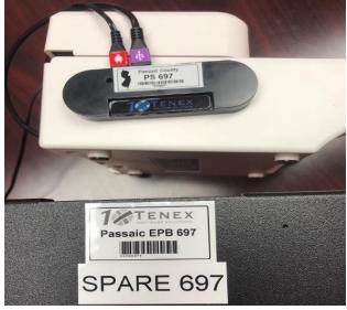
4. Plug in the Print Server. A steady green light indicates the print server is powered on. Plug in the printer power supply (both ends), then turn on the printer.
